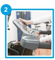
To lift the monitor push the plastic from underneath and pull it up
