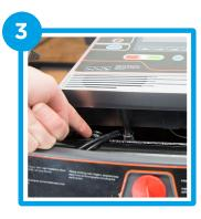
If you struggle, then loosen the two bolts under the monitor
