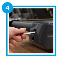
Test the belt after each turn and make sure to reciprocate each turn on either bolt
